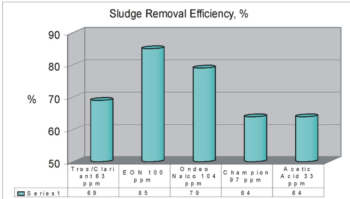
Figure 3. Performance of acid demulsifiers in pilot demonstration tests.
