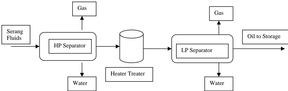
Figure 2. Schematic diagram of Santan Terminal process plant
