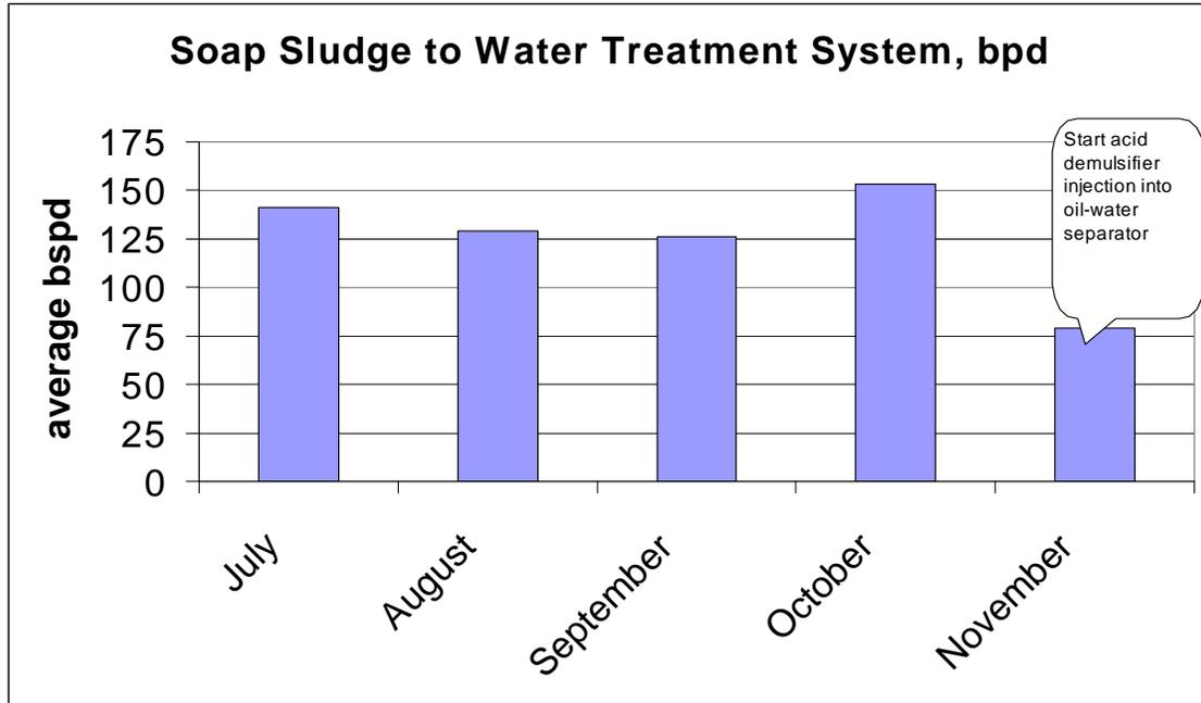
Figure 6. Sludge removal volumes from the water treatment system
