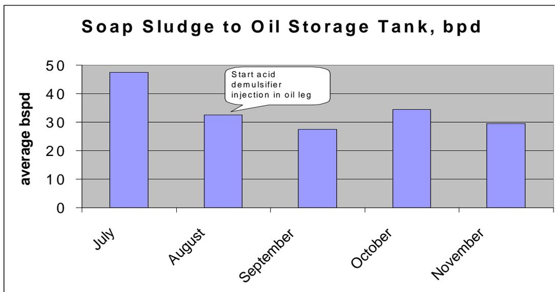
Figure 5. Soap sludge in oil sent to storage
