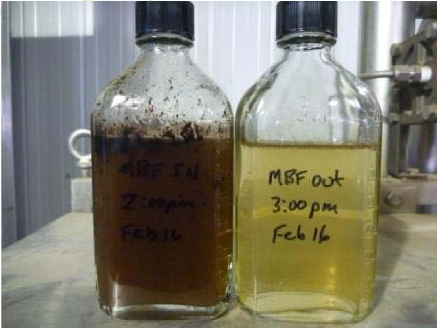
Figure M. Water Samples at inlet and outlet of GFT, Client 2.
