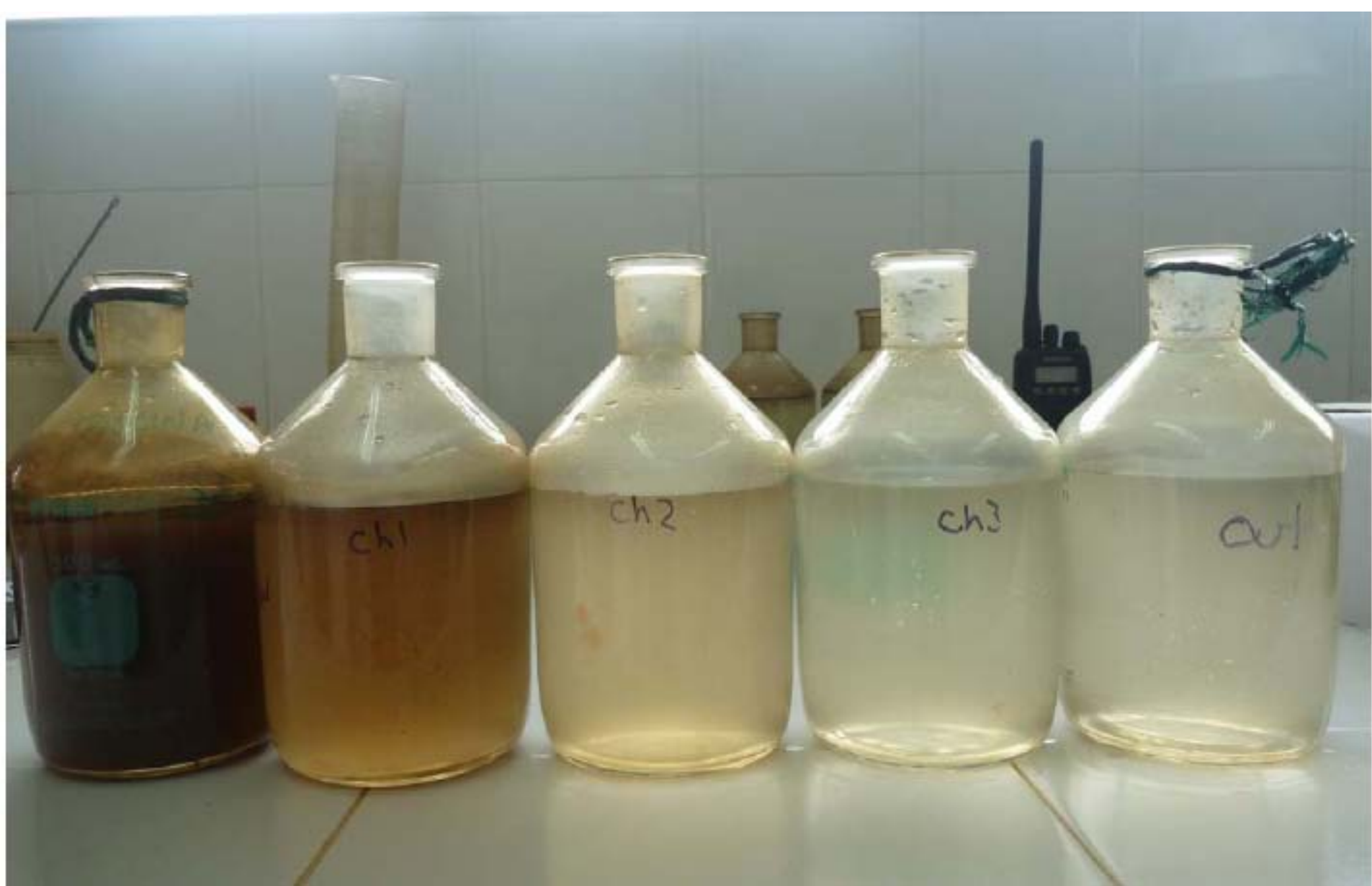
Figure L. Water Samples at the outlet of each chamber collected for Client 1.
