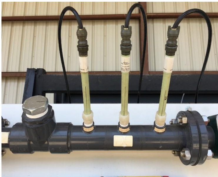
LPR Probes using 304SS, 316SS, and 4130CS electrodes
