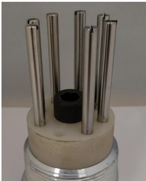
Seven cylinder coupons (4130CS, 4140CS, 4150CS, 4340CS, 17-4SS, 304SS, 316SS)
