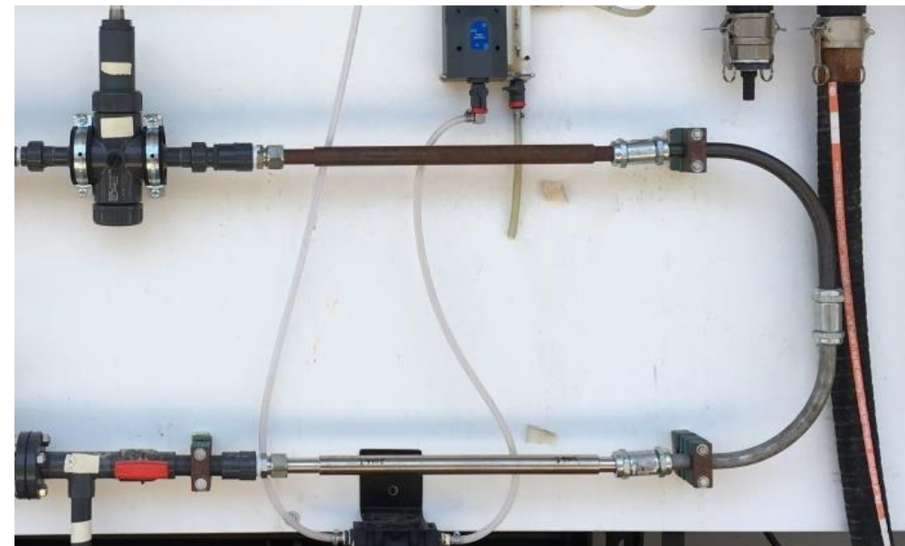
7.3ft of 0.75" ID tubular components (CS, 304SS)
