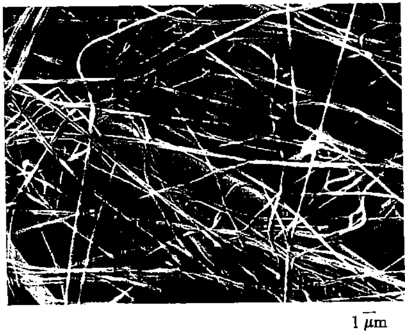
Figure 2 SEM image of nanofibers on larger glass fibers. The nanofibers are made of Nomex™ (tradename of fibers made by the DuPont Company) otherwise known as MPD-I (meta-aramid, poly (meta-phenyleneisophthalamide)).
