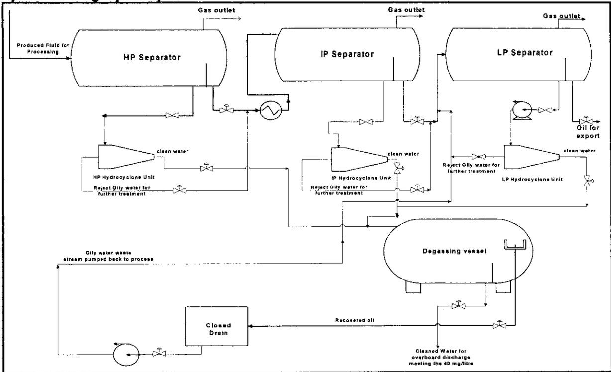
**Figure 2: Typical Produced water treatment facilities for intermediate pressure system using hydrocyclone units**
