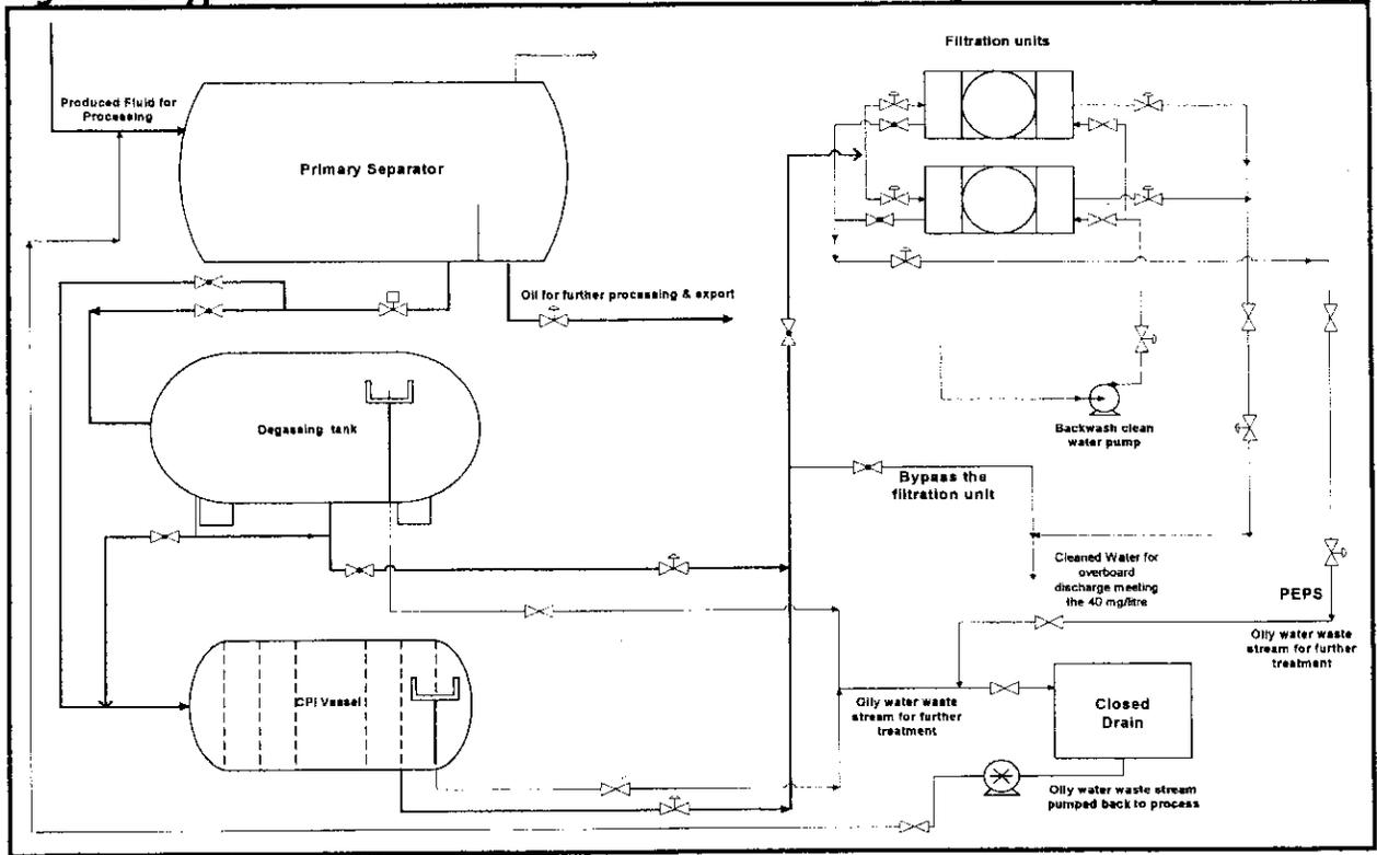
**Figure 6: Typical Produced water treatment facilities using Centrifuge system**
