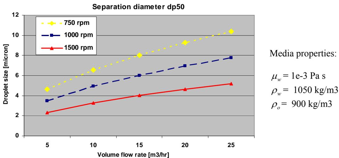
Figure 3: Separation diameter  $dp_{50}$  at different flow rates and velocities.
