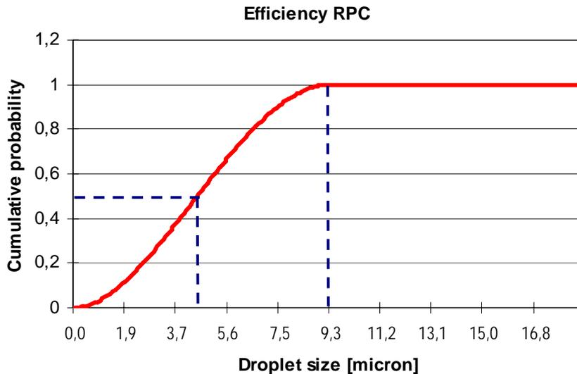
Figure 4: Efficiency of the filter element at 20 m<sup>3</sup>/hr and 1500 rpm.
