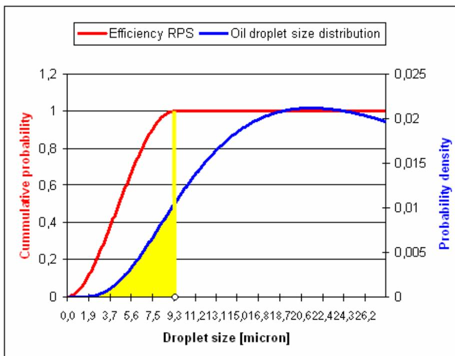
Figure 5: Efficiency with oil droplet size distribution.
