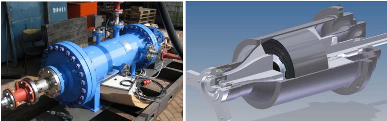
Figure 2: Demo unit Rotational Phase Coalescer
