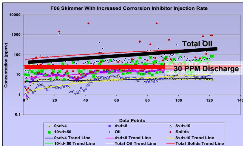
Fig. 5 – ViPA Analysis with Increased CI Injection Rates
