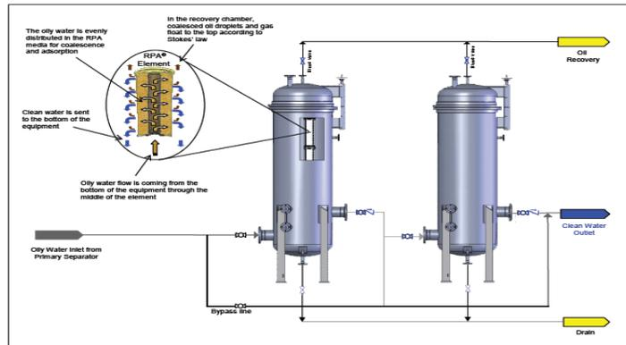
Fig. 6 – General Layout of the Technology
