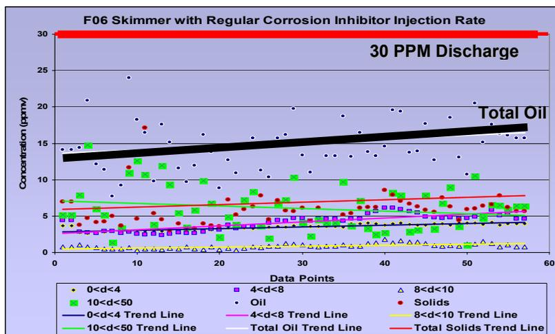
Fig. 4 – ViPA Analysis with Regular CI Injection Rates
