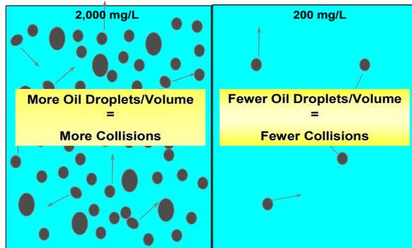
Fig. 1 – Quantity of Oil Droplets per Volume
