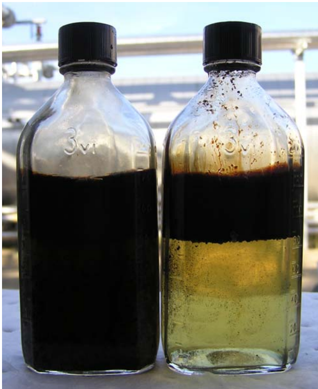
Photograph 1: The novel REB was specifically developed to treat production where a significant amount of the oil produced is carried by the produced water as a reverse emulsion. This particular type of emulsion occurs where high oil production is coupled with high water production, as in SAGD and other high-flow, primary-production fields around the world.
