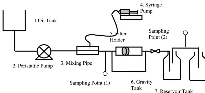
Figure 2: Schematic of Liquid-liquid Coalescence experiment Set-up
