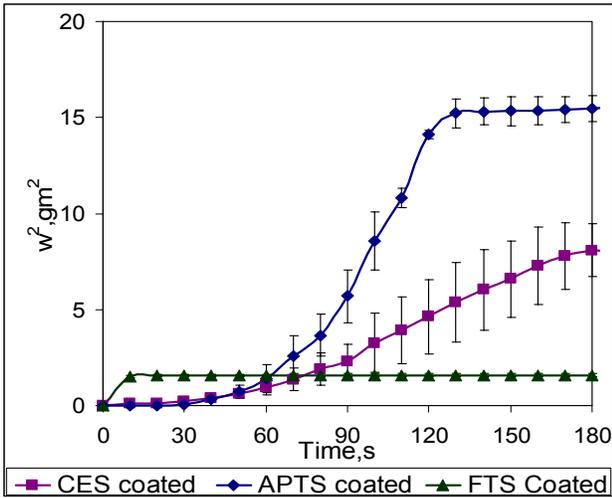
Figure 3: Wetting kinetics for different filter media with water as reference liquid
