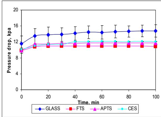
Figure 7: Pressure drop vs. time for the filter media with different coatings. (Each value is an average of the measurements of three filter experiments. The error bars sign standard deviation)
