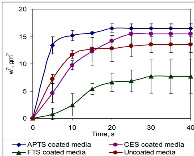
Figure 5: Wetting Kinetics Using Viscor Oil 1487 As A Reference Liquid
