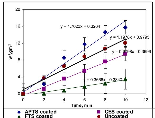
Figure 6: Initial slope of filter media using Viscor oil 1487.
