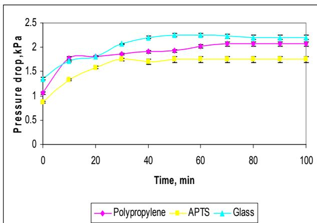
Figure 8: Pressure drop vs. time across the fibrous beds. The error bars show one standard deviation. The data points are the average values of three experiments.
