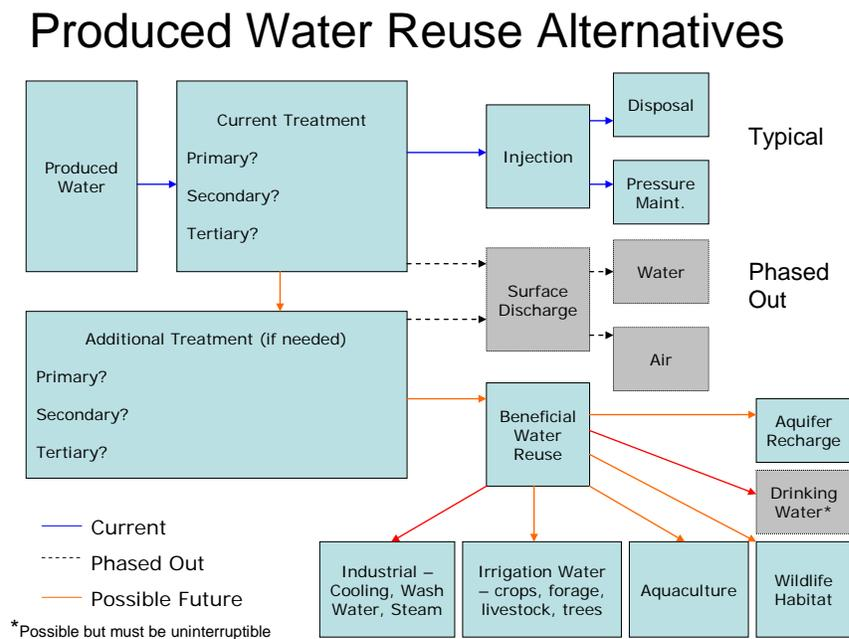
Fig.8-Produced Water Treatment Example PFD
