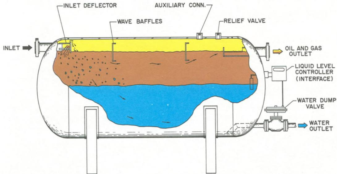
Figure 3: Typical Three-phase separator
