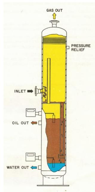
Figure 1 – Typical Vertical Production Separator
