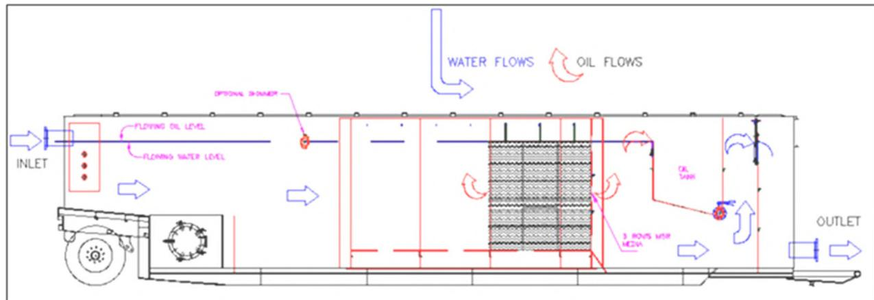
Figure 8: Full-Scale Unit Section
