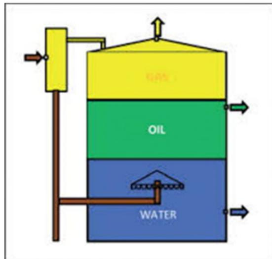
Figure 2: Typical Gunbarrel Separator
