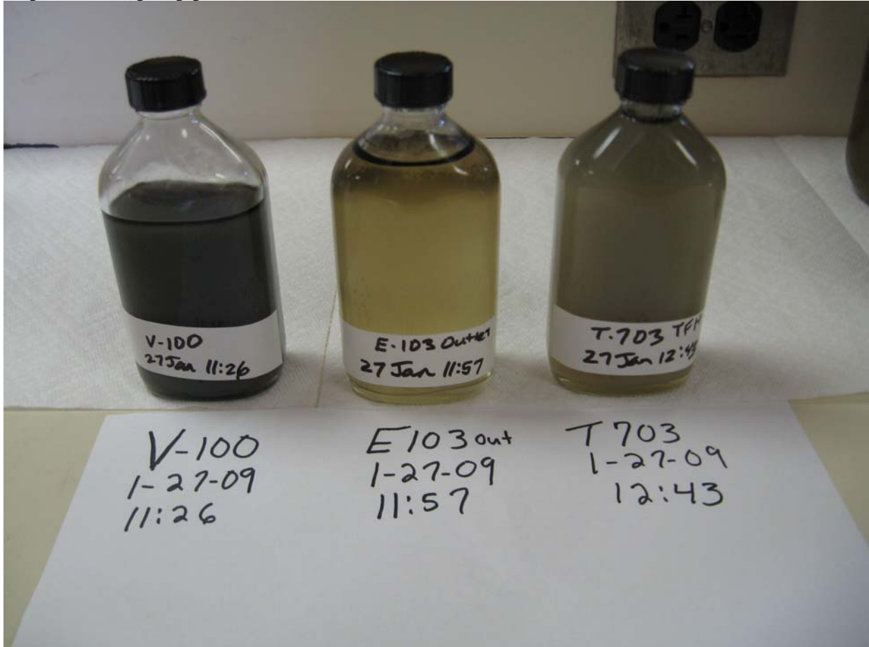
Figure 8: V-100 (Produced Water De-emulsifier), E-103 (Shell side) Sour Water Heat Exchangers and the T-703 (Wastewater Storage Tank) which is immediately upstream of the disposal water pump prior to the well.
