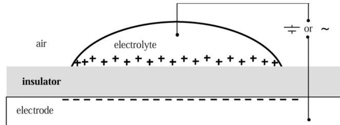
Figure2. The second electrode setup [4].
