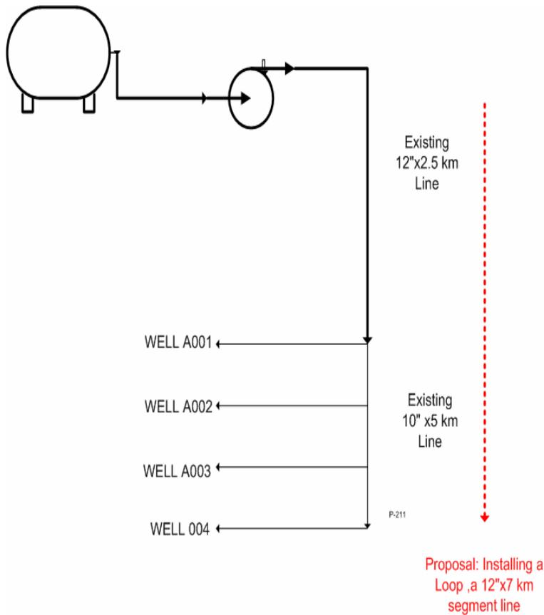
**Case B Plant AX002:** Here is was shown that a problem due to limitation in the pump is looming as the forecast showed that the produced water rate was significantly increasing beyond the existing pump capacity and the injection wells intake, while the flowlines showed no limitations. It was proposed here to install a new pump and a new well.
