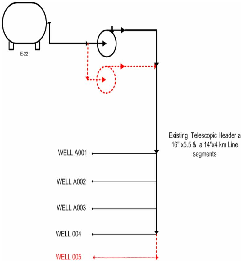
**Case C Plant AX003:** The new injection strategy called for abandoning some injection wells and moving in the field, a distance away from the plant, utilizing watered-out oil wells. Simulation runs showed as the new distant wells were added and old wells close-by were mothballed, severe back pressure would be sustained. The proposed solution was to tie-in to the new wells directly to the system with a dedicated large size diameter .
