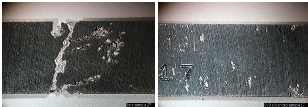
Figure 9: Comparison of 316L coupon (left) and a-Si coupon (right) after ASTM G48 Method B testing. The a-Si coupon shows significantly less corrosion and pitting compared to the 316L coupon.
