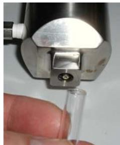
Photo 13. The CT-1000 can accommodate various cuvet sizes and styles.
