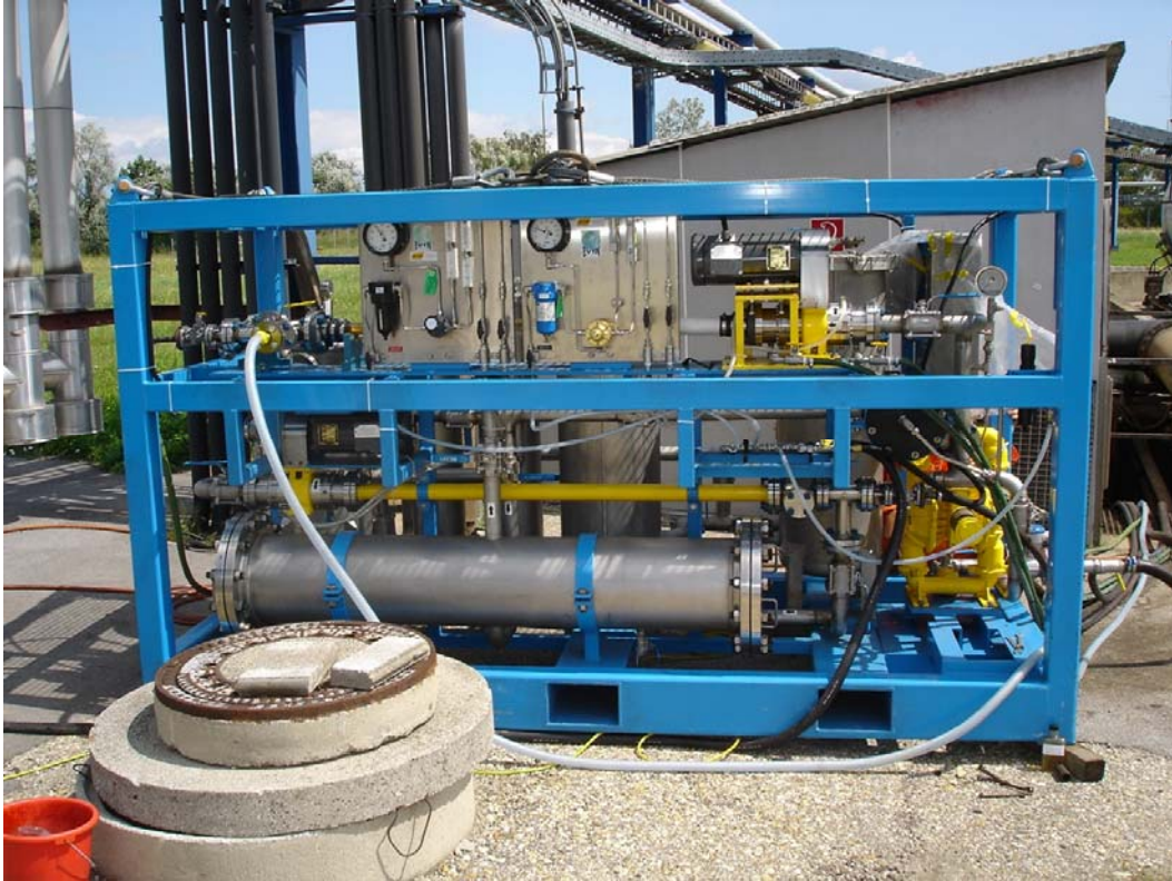
Figure 4 – Voraxial 2000 Separator Skid Test Setup
