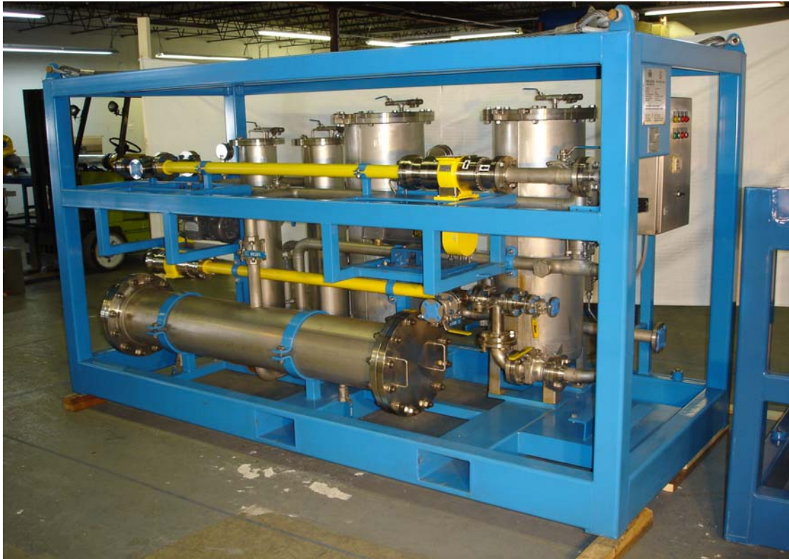
Figure 3 – Voraxial 2000 Separator Skid
