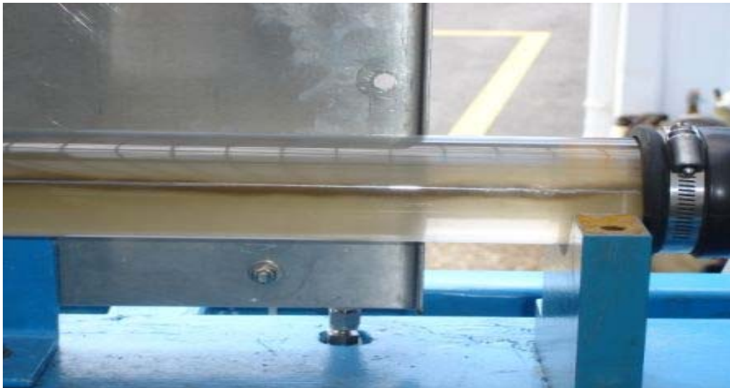
Figure 5 – View of Voraxial Separator Vortex
