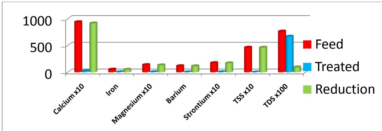
Figure 8 – Concentrations Before and After Treatment
