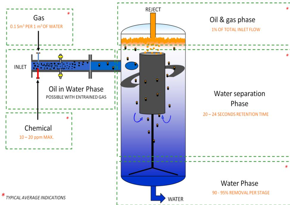
Figure 9 – Compact Flotation Unit
