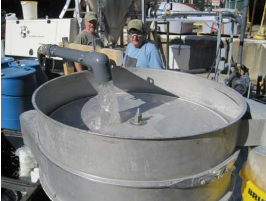
Above: Clean water and spent Osorb after treatment with PW Unit #1.
