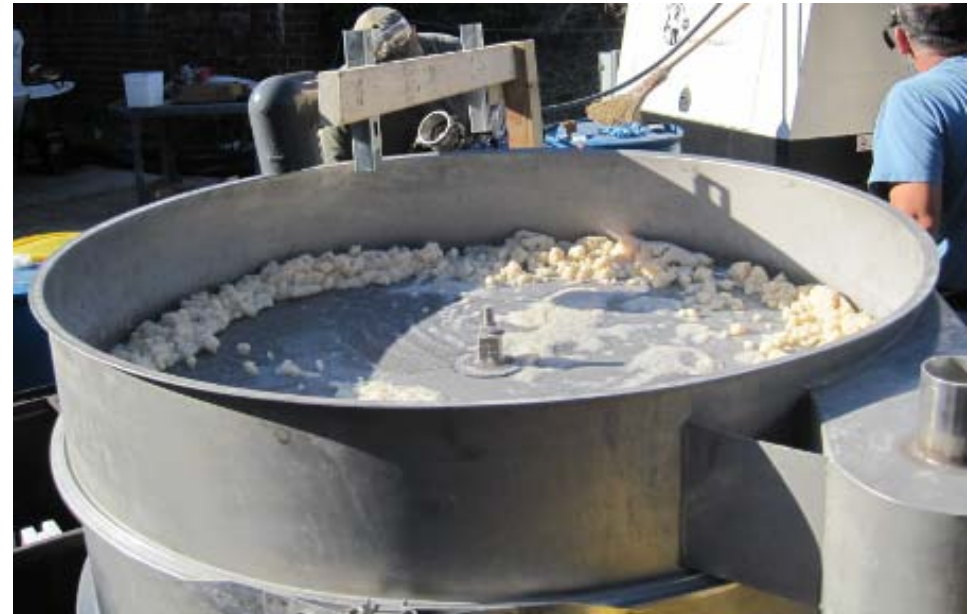
Below: Contaminant-laden Osorb has been separated from the treated water and is ready for regeneration
