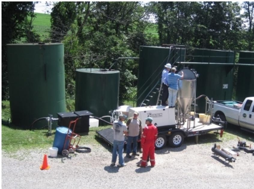
**Figure 5.** Preparation of PW Unit #1 to treat Clinton gas-field produced water.
