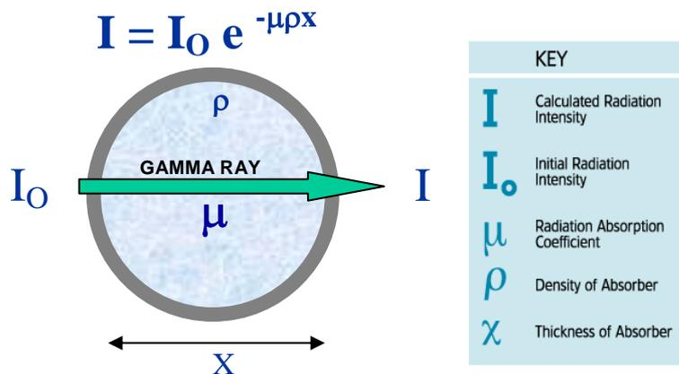
Figure 7 - The Gamma Ray Transmission Equation
