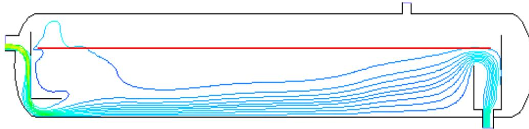
**No Baffles for Flow Control**
