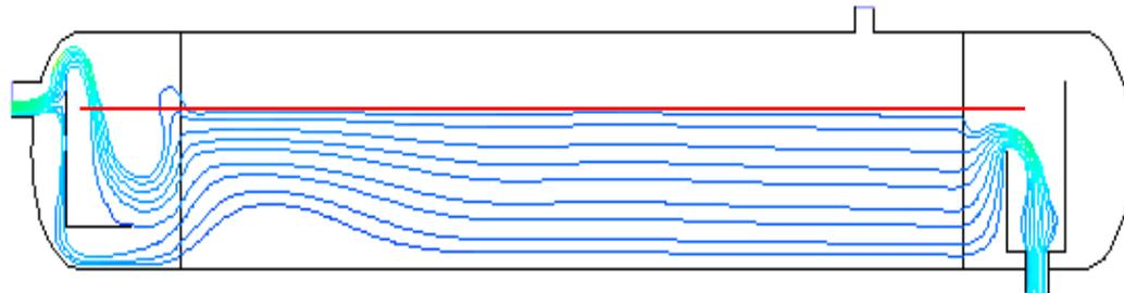
**With Baffles for Flow Control**
